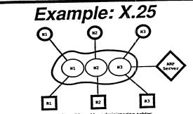
Address resolution on N1 is achieved by administering tables Address resolution on N2 is algorithmic Address resolution on N3 is achived using Directed ARP to an ARP Server
