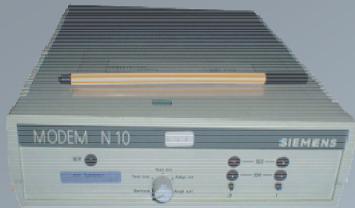
Modem N10 – Siemens 1977 V24, synchron, 9600 Bd
