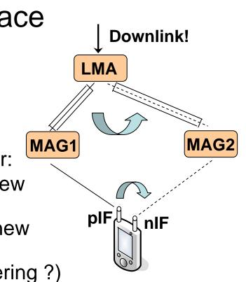
PBU cannot be delayed (nMAG retrieves configuration data for MN) !
