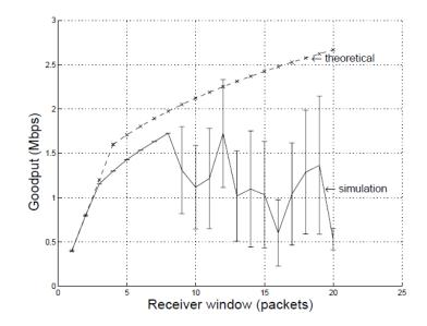
Figure 3: The goodput of the background flow versus the window size with 8 foreground flows, when C = 2000 packets per second, B = 20 packets.
