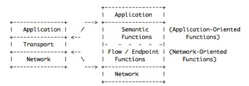
A new location for security functions: between the two functional components
