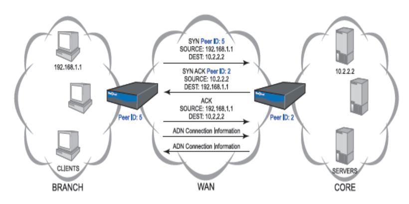
This diagram shows the setup of a Transparent ADN Tunnel
