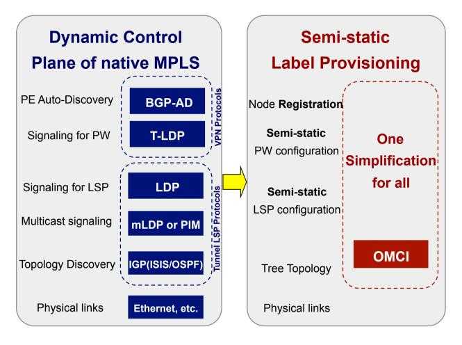
The ONT management and control interface (OMCI) is a management channel between the OLT and the ONUs that supports Ethernet, equipment, subscriber interface, and subscriber feature management.
