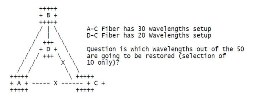
We have WL 1 to 30 setup between C-A, WL 1 to 20 setup between D-C and WL 1-30 already setup between B-C
