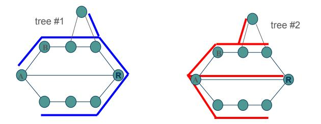
In case of link A-B failure, the notifications originated on node B will reach R on tree #1 and get replicated on the tree#2 while notifications originated on node A will reach R on tree #2 and get replicated on the tree#1
