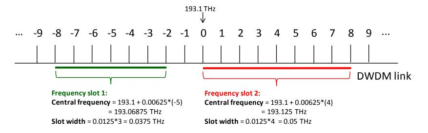
Flexi-Grid: a new WDM frequency grid defined with the aim of allowing flexible optical spectrum management, in which the Slot Width of the frequency ranges allocated to different channels are flexible (variable sized).
