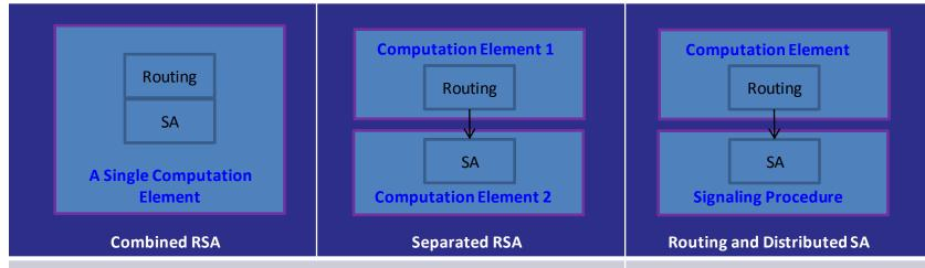
Both of the route and frequency slot are determined before the signaling procedure. With Separate RSA, Routing may suggest candidate frequency slot to SA which will allocate final slot assignment from the candidate pool.
