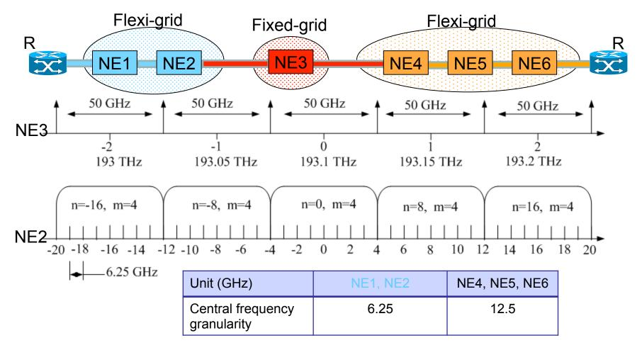
Configure the flexi-grid nodes in such a way that the central frequencies and slot width parameters are backwards compatible with the fixed DWDM grids:
