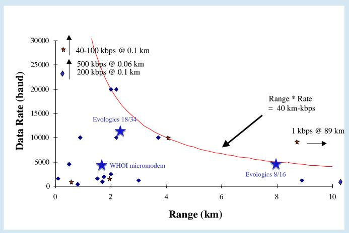
Image from: "The state of the art in underwater acoustic telemetry"
