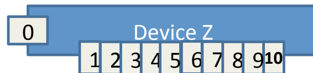
PDU w/ one inlet and 10 outlets
