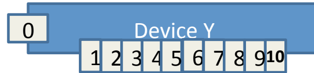
PDU w/ one inlet and 10 outlets
