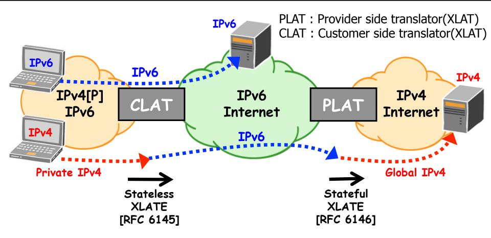
464XLAT provides limited IPv4 connectivity across an IPv6-only network by combining existing and well-known stateful protocol translation RFC 6146 in the core and stateless protocol translation RFC 6145 at the edge.
