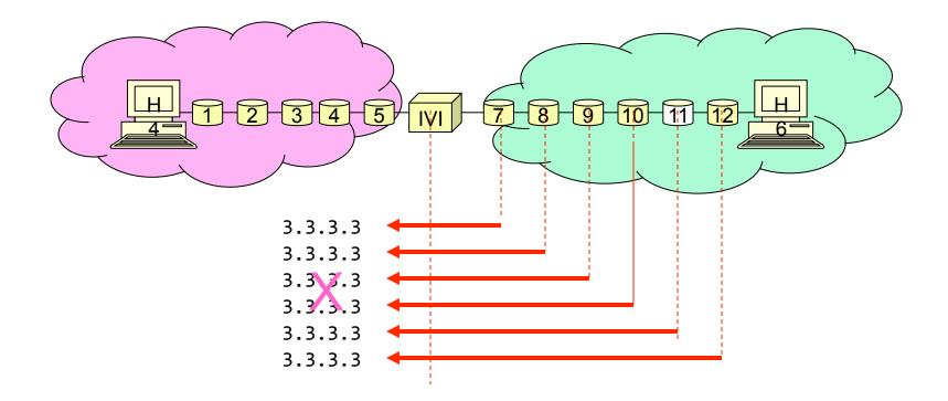
IPv4 recipient of the ICMP message should be able to distinguish between different IPv6 ICMPv6 origination → needs a pool
