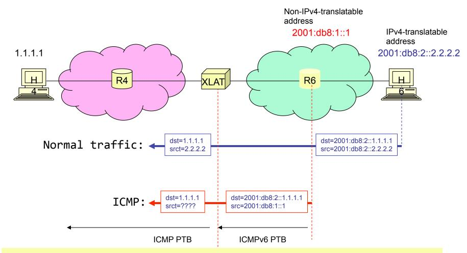
RFC6145: The IPv6 addresses in the ICMPv6 header may not be IPv4translatable addresses. ... A mechanism by which the translator can instead do stateless translation is left for future work.
