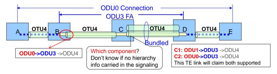
• If only bundle homogeneous component links, ERO can indicate the last TE link
