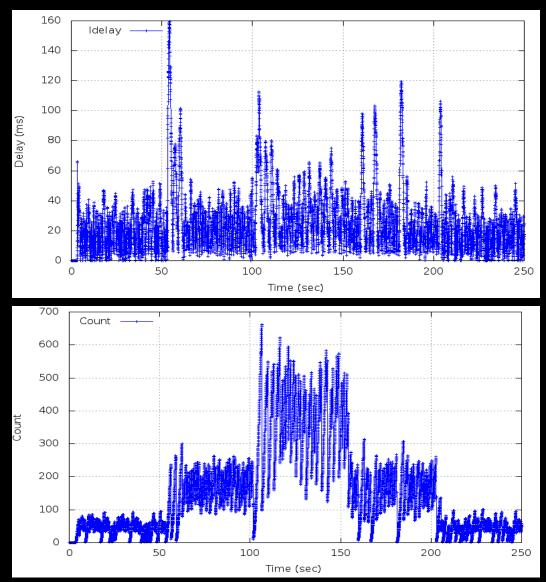
CoDel does not work well under heavy load. Their control parameter, count, oscillates widely under those situations. The feedback loop is not stable.
