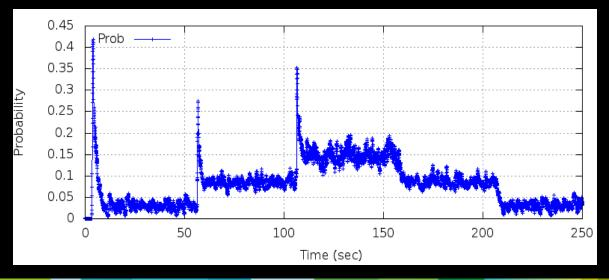
Regardless of traffic intensity, PIE keeps latency around the target value by adjusting drop probability accordingly. The feedback loop is in tight control.
