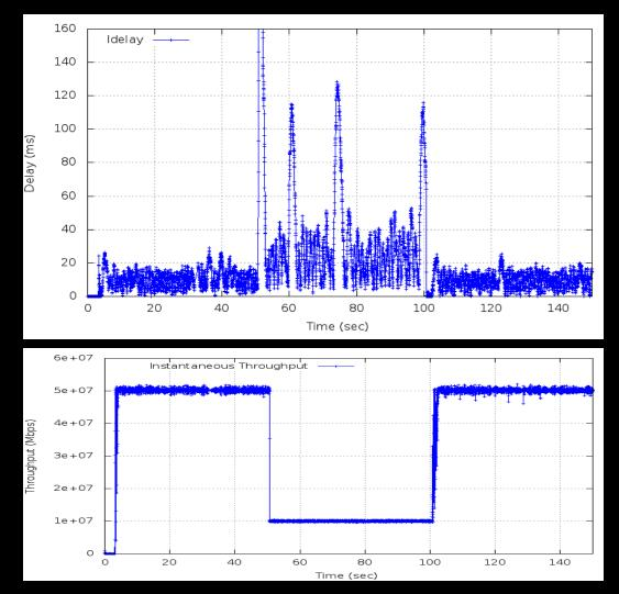
When the queue draining rate dips from 50Mbps to 10Mbps, CoDel can't keep the latency low throughout the process
