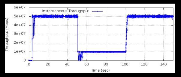
When the queue draining rate dips from 50Mbps to 10Mbps, PIE is able to keep the latency low throughout the process
