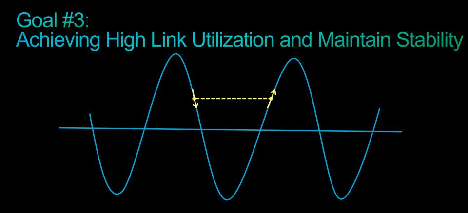
Traditionally drops/marks increase as the queue lengths increase (longer delays), which could result in wide swing delay variation
