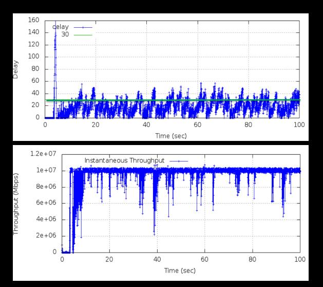
Under low load case, TCP Sawtooth is observable. However, PIE can regulate TCP flows so well that the link is close to full capacity while maintaining low latency
