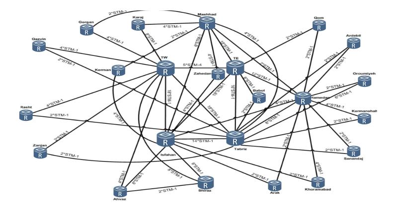
Large Network with a lot of MPLS-TE Tunnels requires massive configuration work. The operation is not only time consuming but also prone to mis-configuration for Service Providers.
