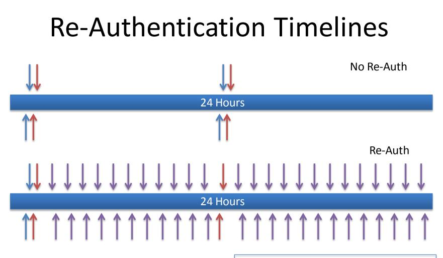
Assumptions: Loosely coupled authentication/authorization, mapping lifetime is 24 hours, key lifetime is one hour.
