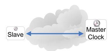
Slave is connected to a single master using a single path, e.g. PTP.
