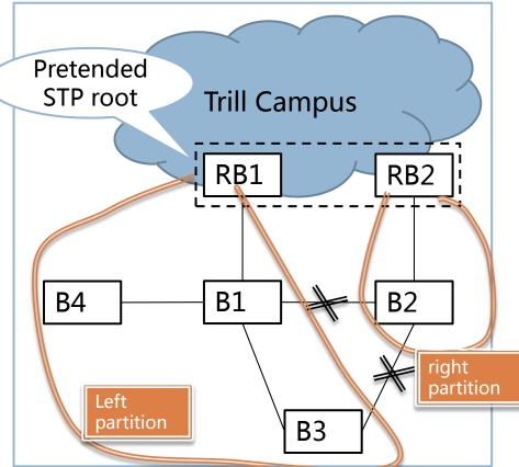
Method 2 (Ethernet LAN Partition approach): •RB1 & RB2 pretend to be single STP root •Make Ethernet LAN domain partitioned •Achieve per-vlan load balancing. AF & its inhibition timer no longer not necessary
