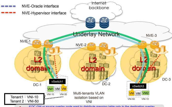
Local source NVE translate destination MAC address of ARP from source Tenant system to its own MAC address, forward it to destination tenant system and populate mapping table corresponding to destination NVE with received ARP reply.
