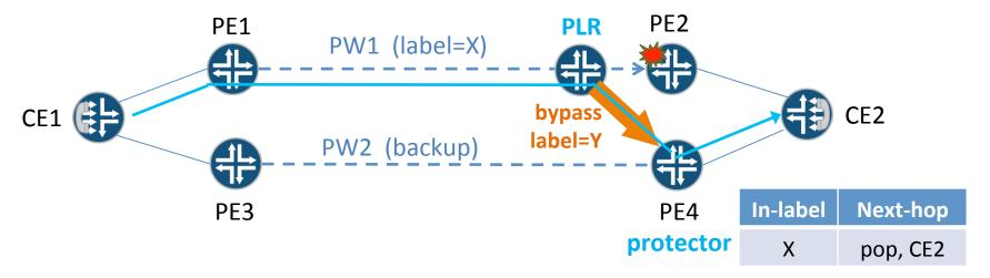
PLR is the penultimate hop router. It has established a bypass to protector (PE4). Protector (PE4)
