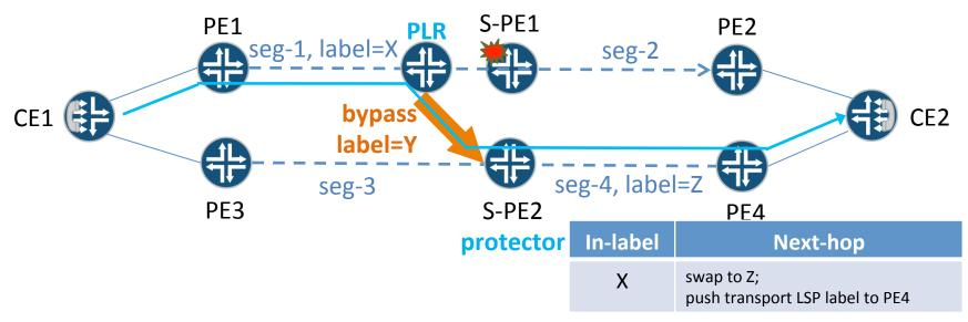
PLR is the penultimate hop router of seg-1. It has a bypass to protector (S-PE2). Protector (S-PE2)
