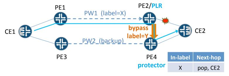
PLR is the primary PE (PE2). It has established a bypass to protector (PE4). Protector (PE4):
