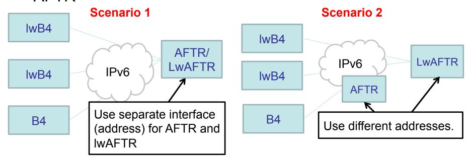
B4 and lwB4 must be configured with different tunnel endpoint addresses.
