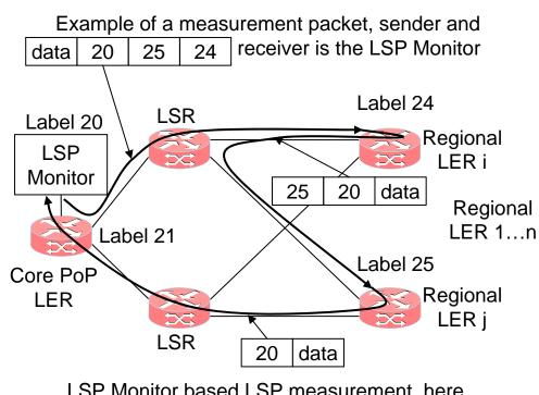
LSP Monitor based LSP measurement, here with 3 LSP segments
