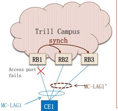
> Manual provisioning inconsistency: may cause frame loss. Auto discovery required?
