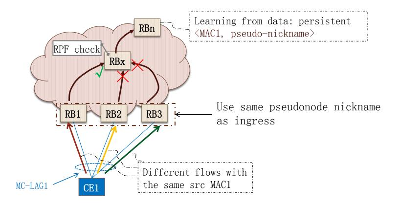
Psedunode nickname was meant to solve previous two problems, however it introduced another issue: dropping due to RPF check on multi-destination data
