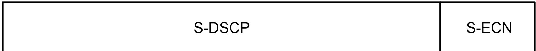
Sender DSCP and ECN field format
