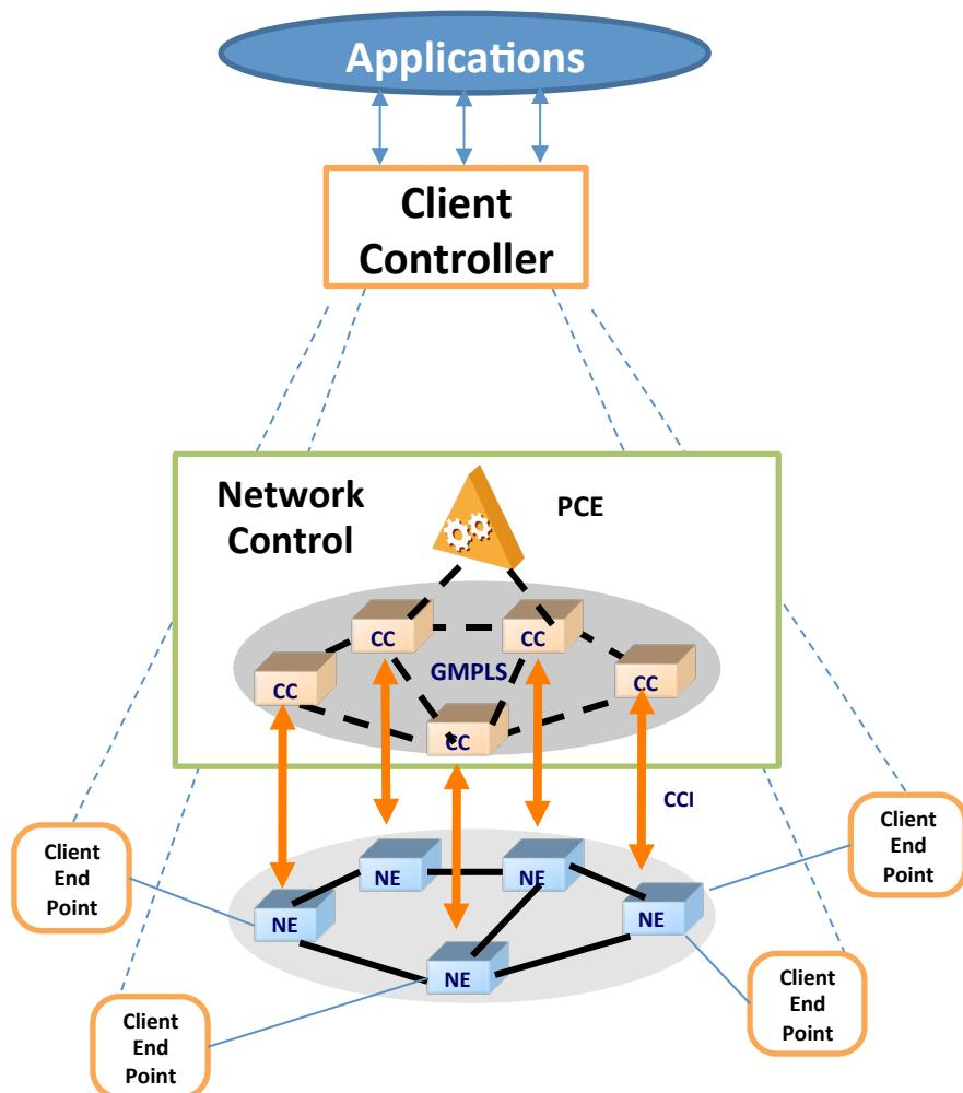
**But current GMPLS/PCE architecture does not support programmable interfaces for network virtualization**
