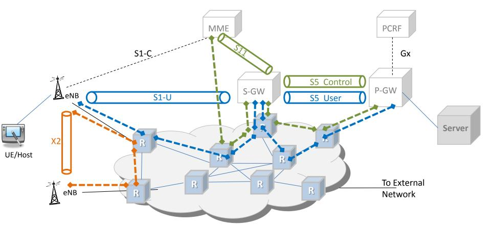
More than 1 tunnel between policy enforcement points. Example: UE PDN connection traverses [eNB] << S1-U >> [SGW] << S5/S8 >> [PGW].
