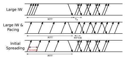
Time diagram for a transmission of 12 segments
