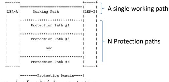
Example of multi-failure protection
