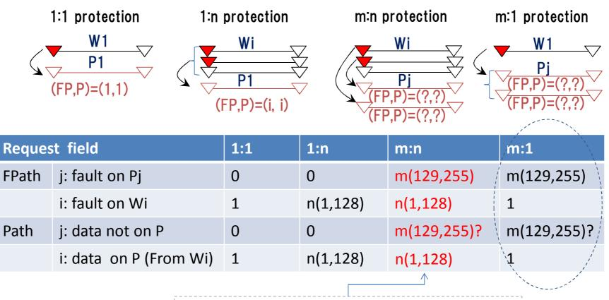
m:n protection can be implemented by software, but <u>difficult to be implemented by hardware</u>, because a huge number of state machines need to be managed.
