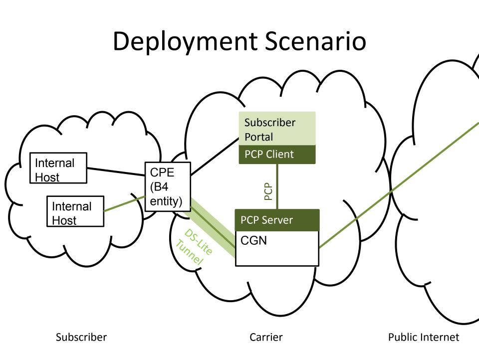
Subscribers can freely choose their internal IP addresses: This potentially leads to overlapping IP address spaces.
