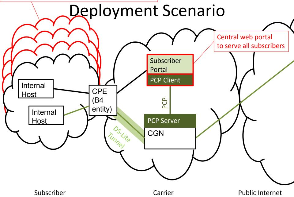
Subscribers can freely choose their internal IP addresses: This potentially leads to overlapping IP address spaces.
