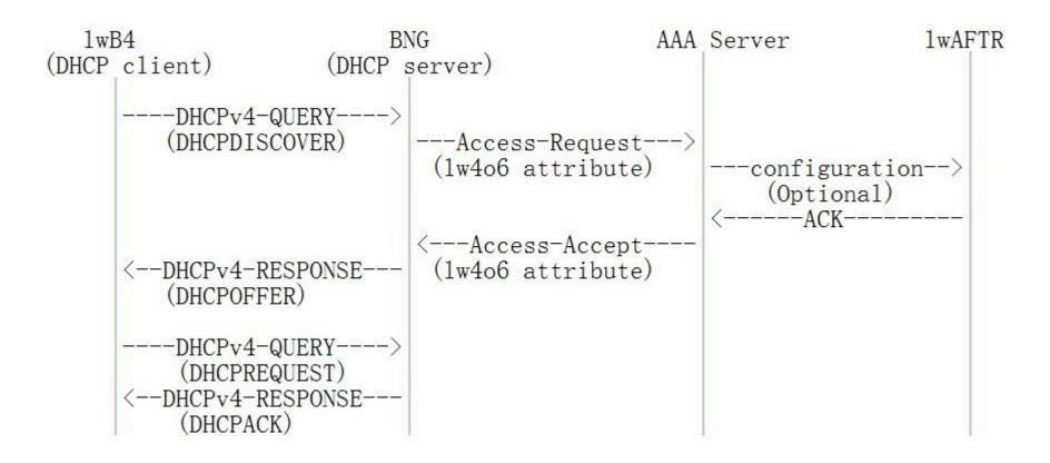
If the mapping tables are created dynamically by AAA server, AAA configures lwAFTR by [I-D.zhou-dime-4over6provisioning] or COA requests [RFC5176]
