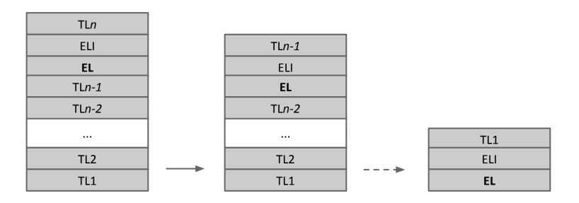
EL is **re-used after pop** by pushing below next label Label operation changes, but end-to-end flow is consistently identified with <u>single EL</u> EL is at a shallow depth along entire path.
