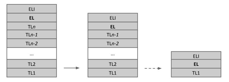
EL is pushed on top of label stack. EL is **re-used after pop** by pushing on <u>top</u> of next tunnel label Label operation changes, but end-to-end flow is consistently identified with <u>single EL</u> EL is at a shallow depth along entire path.
