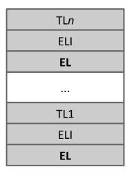
Label stack depth is **three** times the number of tunnel labels
