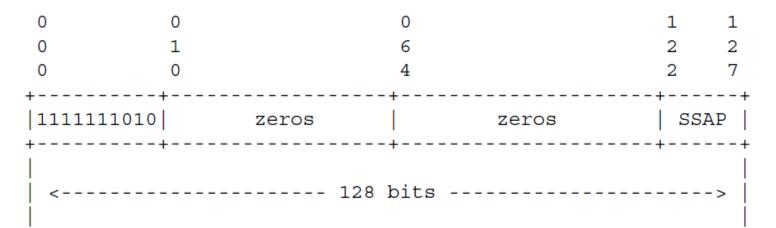
Figure 4: IPv6 link-local address in NFC
