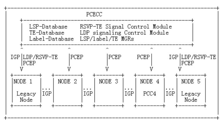
Global and local labels are negotiated and assigned for tech nodes in the network through PCE central controller.
