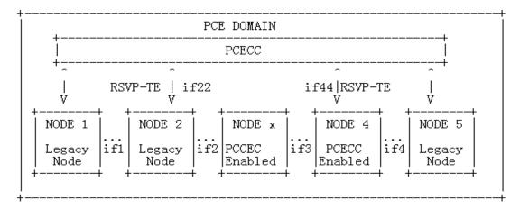
□ In this example, there are five nodes for the TE LSP from head end (node1) to the tail end (node5), where the nodes between node2 and node4 are represented as Node-X are central controlled and other nodes are legacy nodes.
