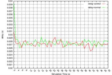
Average e2e delay: In case of tunnel control: 0.027071s. In case of no tunnel control: 0.027615s.
