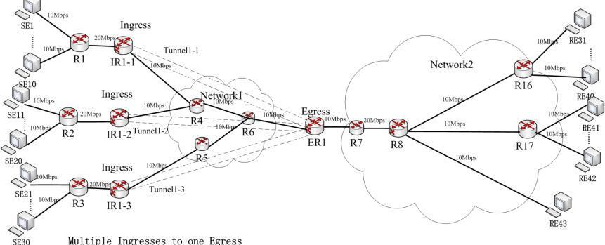
Testbed: NS3. SEx: Sender, Rate: 1Mbps. IR1-x: Tunnel Ingress. Rx: Router, ECN-enabled. Manager action: Random Drop. IPFIX is used for congestion information feedback.
