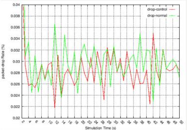
Average packet loss: In case of tunnel control: 0.028127%. In case of no tunnel control: 0.029859%.
