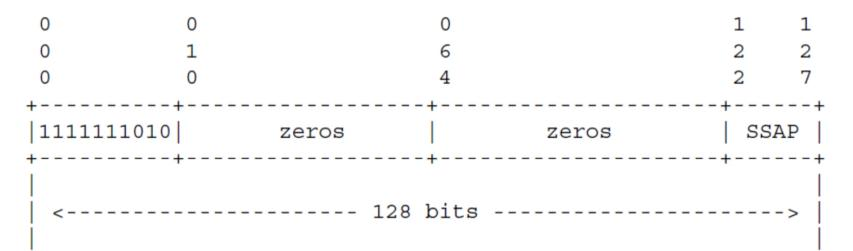
Figure 4: IPv6 link-local address in NFC
