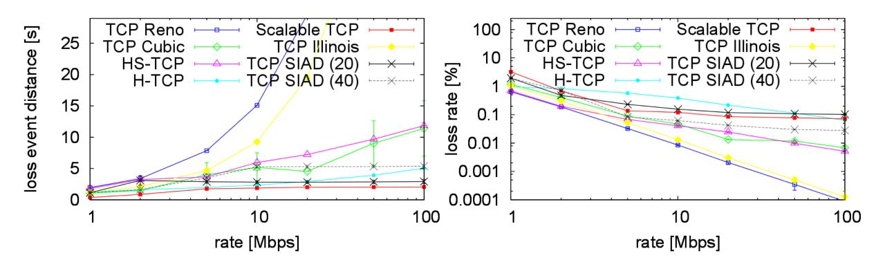
→TCP SIAD induces fixed feedback rate independent of link bandwidth
