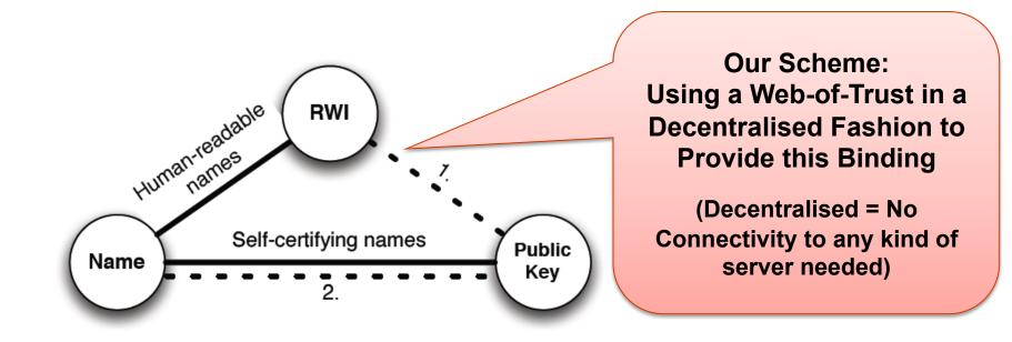
Figure 1: A depiction of the three entities and the different bindings between them. Two naming schemes provide different intrinsic bindings (solid lines) but require both an external authority to provide one additional binding (dashed line): with self-certifying names it's the binding (1), whereas with humanreadable names it's the binding (2).
