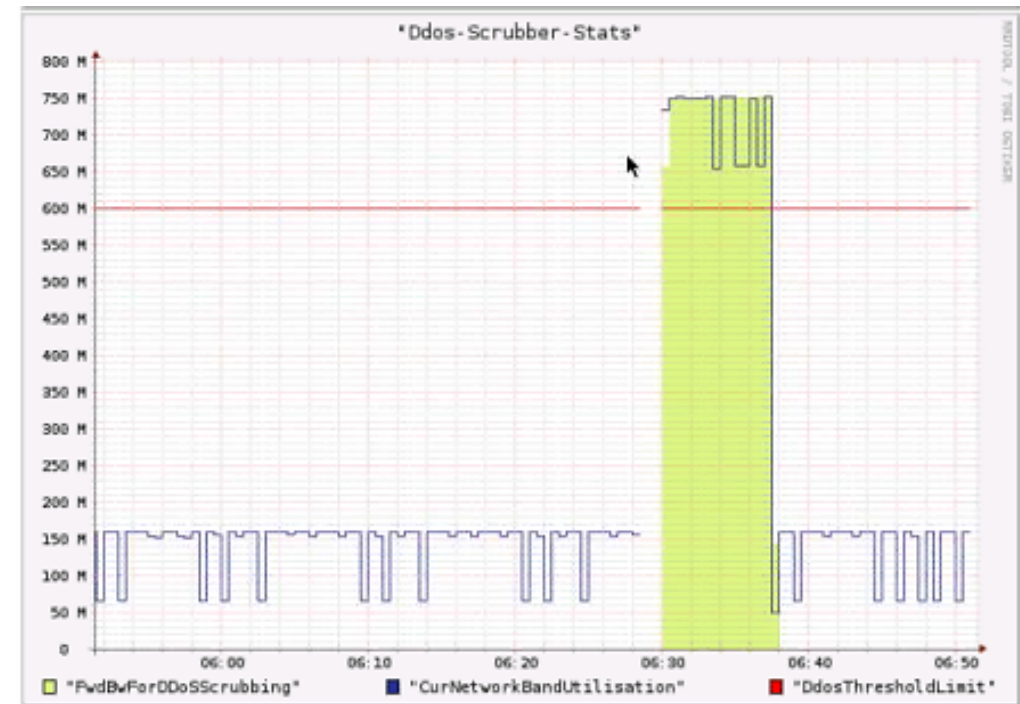
DDoS Scrubber inserted when Traffic Spikes over 600 Mb/s Threshold
