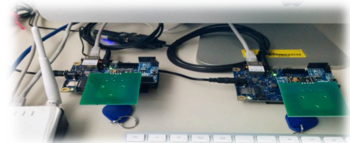
Intel Galileo board with Debian Linux OS
