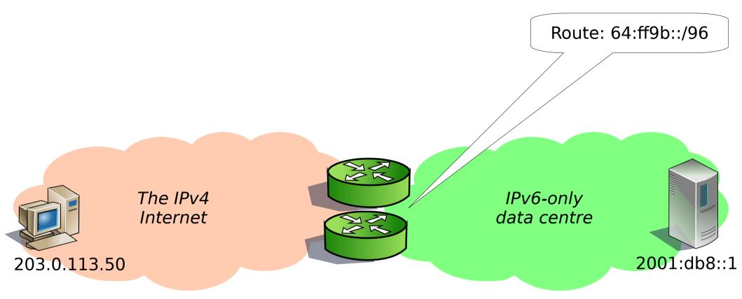
An IPv6 /96 prefix is assigned as the translation prefix representing the IPv4 internet and routed to the SIIT-DC gateways
