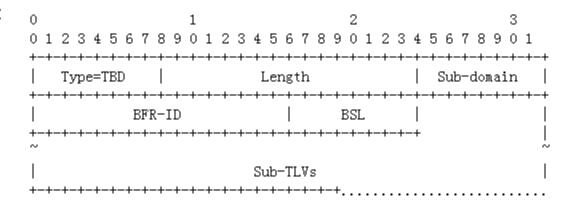
■ MPLS-BIER Encapsulation sub-TLV is a sub-TLV of the BIER TLV encoding the MPLS-BIER specific information.
