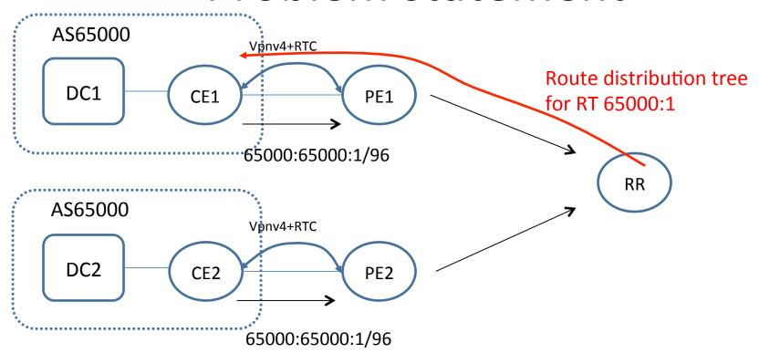
When disjoint ASes setup is used, route distribution tree is wrongly built, preventing communications between sites
