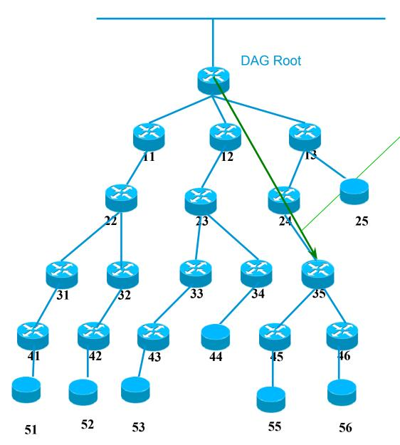
Adding New (projected) DAO with path segment unicast to target 56 via 13 (ingress), 24, and 35 (egress)
