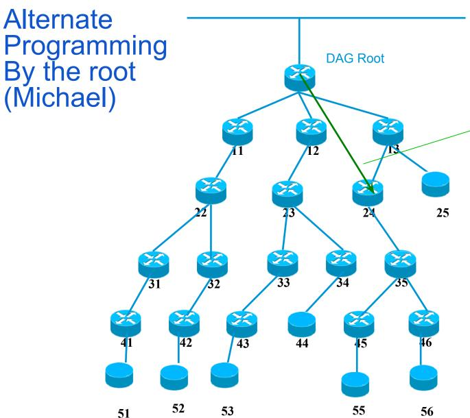
ALT: Adding New (projected) DAO with path segment unicast to target 35 via 13 (ingress) and 24 (egress)
