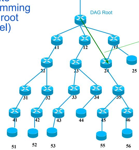
ALT: Adding New (projected) DAO with path segment unicast to target 35 via 13 (ingress) and 24 (egress)
