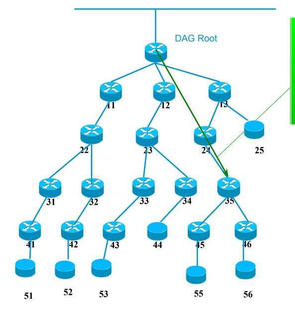
Adding New (projected) DAO with path segment unicast to target 56 via 13 (ingress), 24, and 35 (egress)
