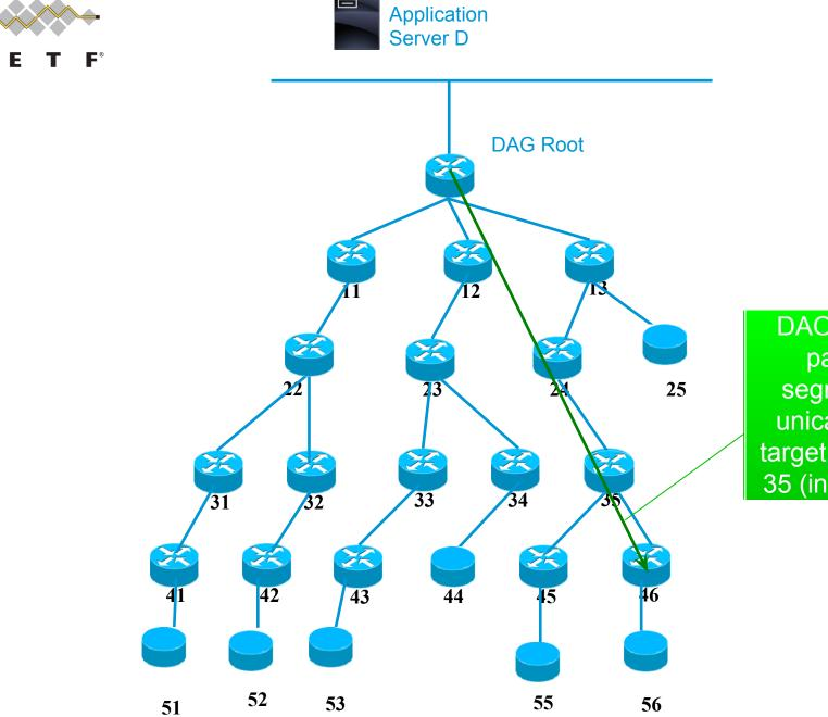
DAO with path segment unicast to target 56 via 35 (ingress)
