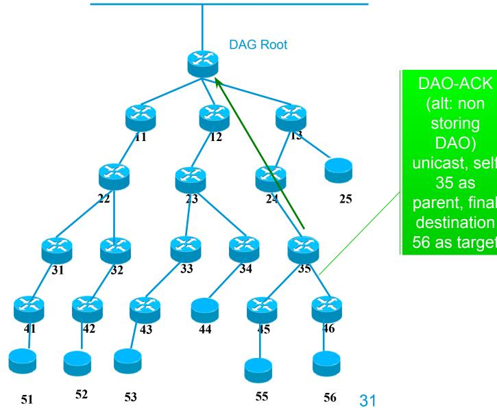
(alt: non storing DAO) unicast, self 35 as parent, final destination 56 as target
