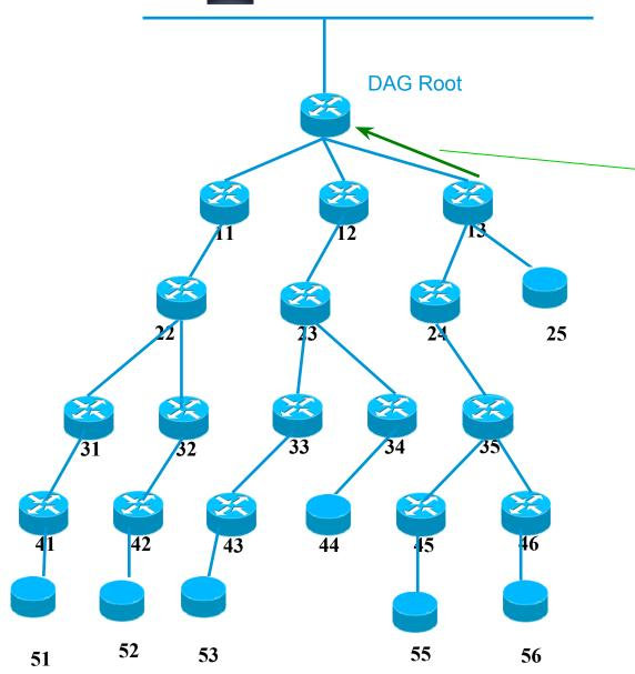
DAO-ACK (alt: non storing DAO) unicast, self 13 as parent, final destination 56 as target
