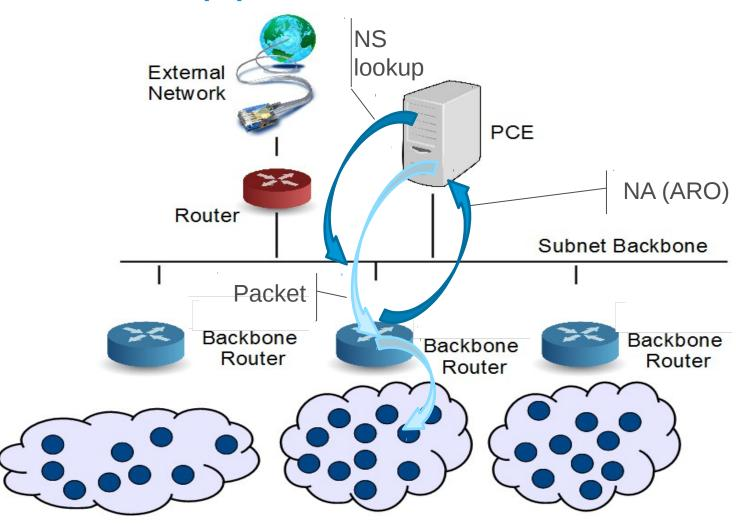
Mixed mode ND BBR proxying over the backbone **Enabling Next-Gen** backbone
