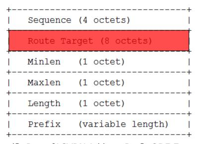
Type Specific Part of L3VPN Address Prefix ORF Entry Encoding
