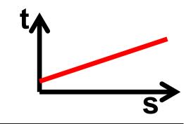
$Delay = d_0 +$ PacketSize / LinkCapacity
