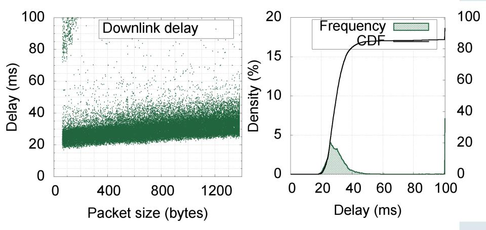
Details: random 50K packets, 64-1400 bytes, i.p.delay 100-5000 ms (total 36 hrs)
