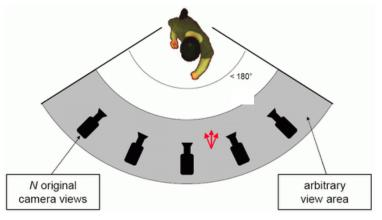
Multi-view video consists of multiple views taken by multiple cameras from different positions and angle.
